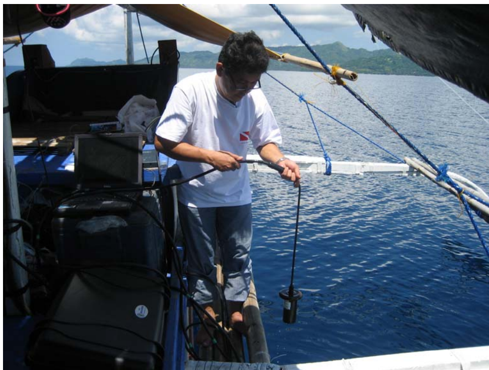
Figure 3.1 : Ramon Cruz of the University of the Philippines in the Visayas, In-situ sampling with the Wet Labs ECO-FLRT Fluorometer.
